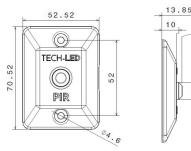
TECH-LED PIR DIR Ideal for commercial and specialist vehicles, the PIR-000 switch units can be used to convert any vehicle accessories that require PIR activation, regardless of who made it.
