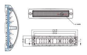
The Cylon is a high-intensity, ECE Regulation 65 approved, warning lamp suitable for use in a variety of commercial applications. Offering multiple fixing methods and incorporating high-quality materials, the Cylon also offers robust durability, making this product highly versatile for both vehicle builders and operators.
